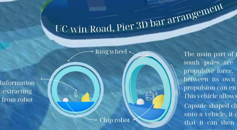
The main part of the system is the vertical magnet ring. On this ring, the north and south poles are placed alternately, balancing the gravitational force and the propulsive force. As the vehicle moves through the magnetic field, the interaction between its own magnetic elements and magnetic fields generates thrust. This propulsion can either attract or repel the vehicle, allowing for controlled movement. This vehicle allows the vehicle to travel in any kind of direction.
